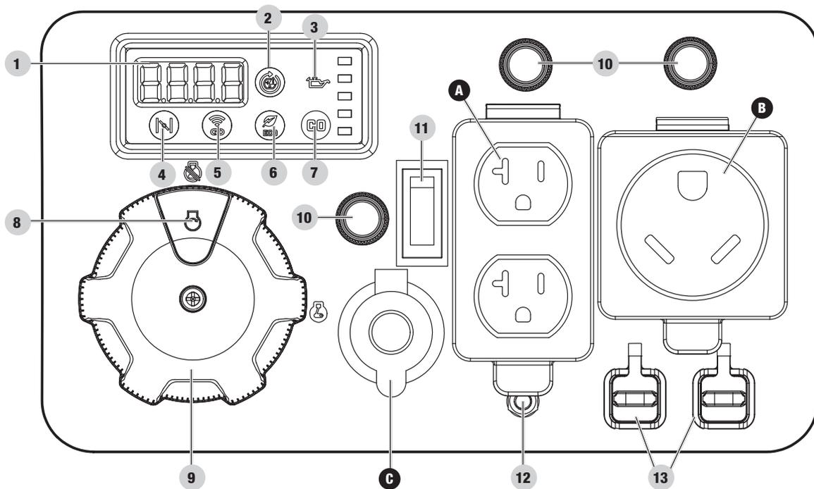
1. **Intelligauge with Power Meter** – Four mode digital meter for displaying run time, total time, voltage, hertz and power output.
