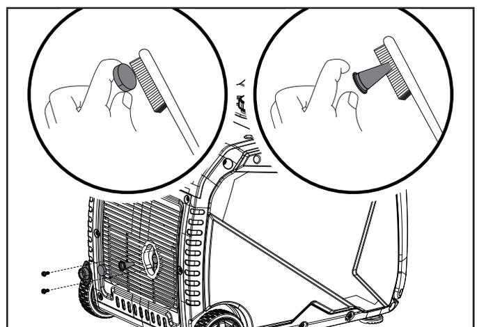
5. Replace the spark arrestor and spark arrestor screen if it they damaged.
