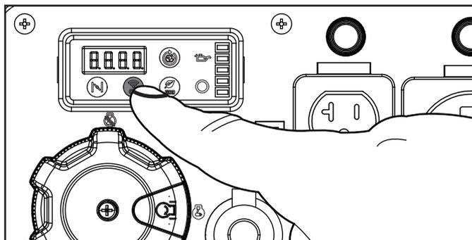
4. Push and release the STOP button on the remote key fob. The blue LED on wireless set button will blink once to indicate program is erased and generator is ready for pairing.
