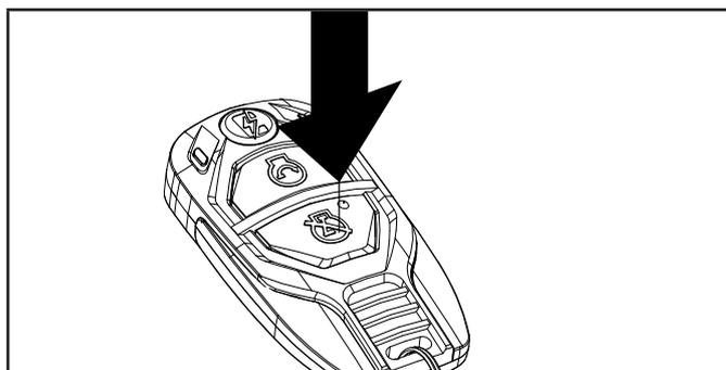
5. Push and release the START button on the remote key fob. The blue LED on wireless set button will blink once to indicate the remote has been programmed.
