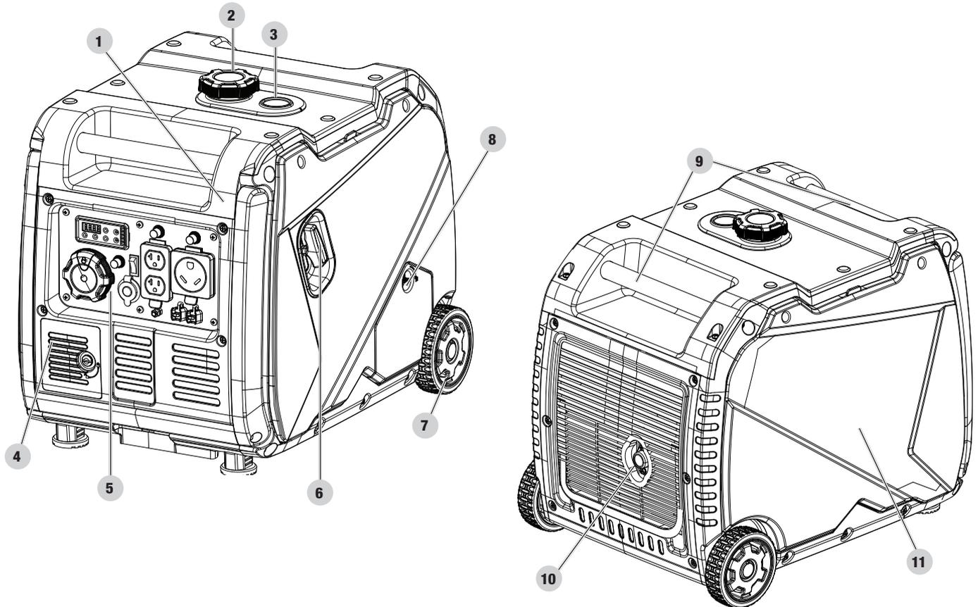
1. **Folding Handle** – Used to move unit by lifting and rolling on wheels. Do not use to lift or carry the unit.
