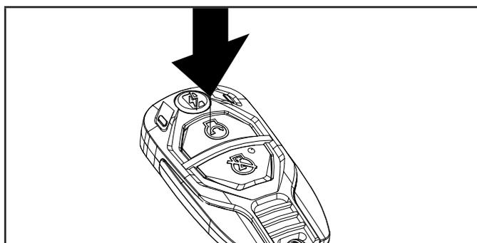
6. Push and hold the wireless set button approximately three seconds until the blue LED on wireless set button turns off.
