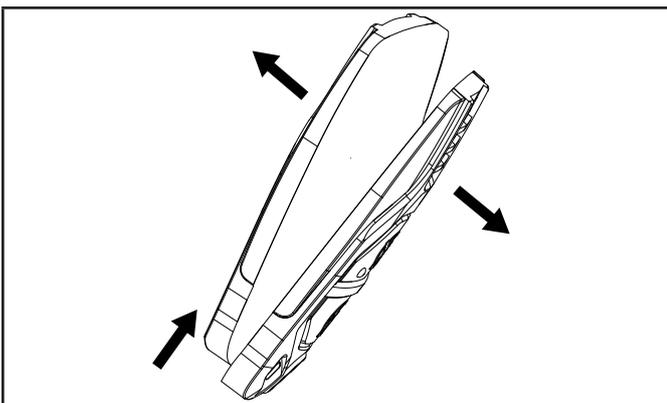
5. Carefully remove the circuit board to locate and replace the CR2016 battery.
