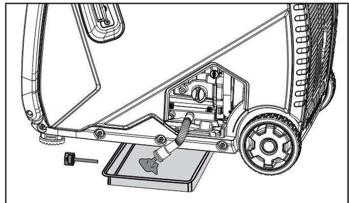
5. Replace the oil drain plug.
