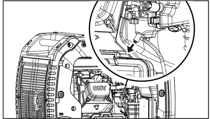
6. When gasoline stops flowing from the clear tube, rotate drain screw clockwise until tight. Properly dispose of the drained gasoline according to local regulations or guidelines.
