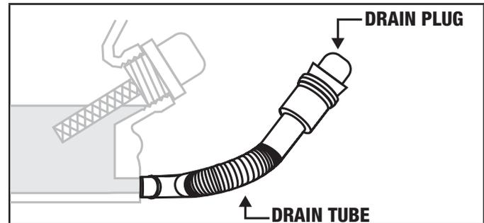
4. Ensure the oil drain hose is lower than the engine and allow the oil to drain completely into an appropriate container.
