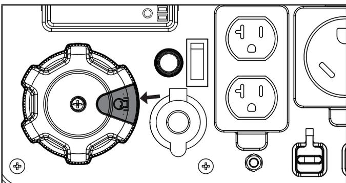
6. Do not over-choke. As soon as engine starts, push the choke button one time to set the choke to the "RUN" position. Choke button will no longer be illuminated when in "RUN" position.
