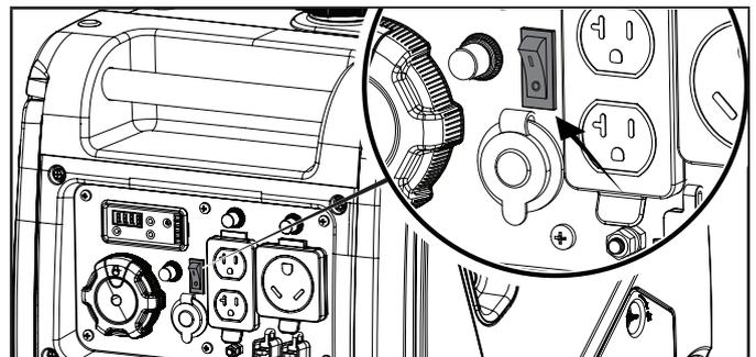
**Important:** Always ensure that the EZ Start Dial and battery switch are in the "OFF" position when the generator will not be used for an extended period of time.
