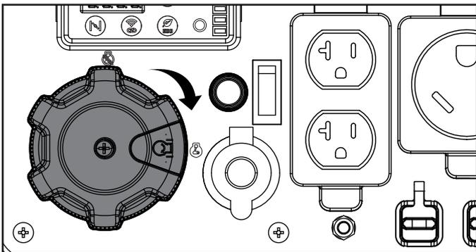
4. Push the choke button one time to set the choke to the "CHOKE" position. Choke button will illuminate when in "CHOKE" position.
