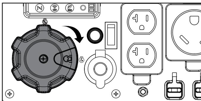
2. Turn the battery switch to the "ON" position.
