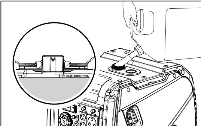
3. The approximate fuel level is shown on the fuel gauge on top of the fuel tank.
