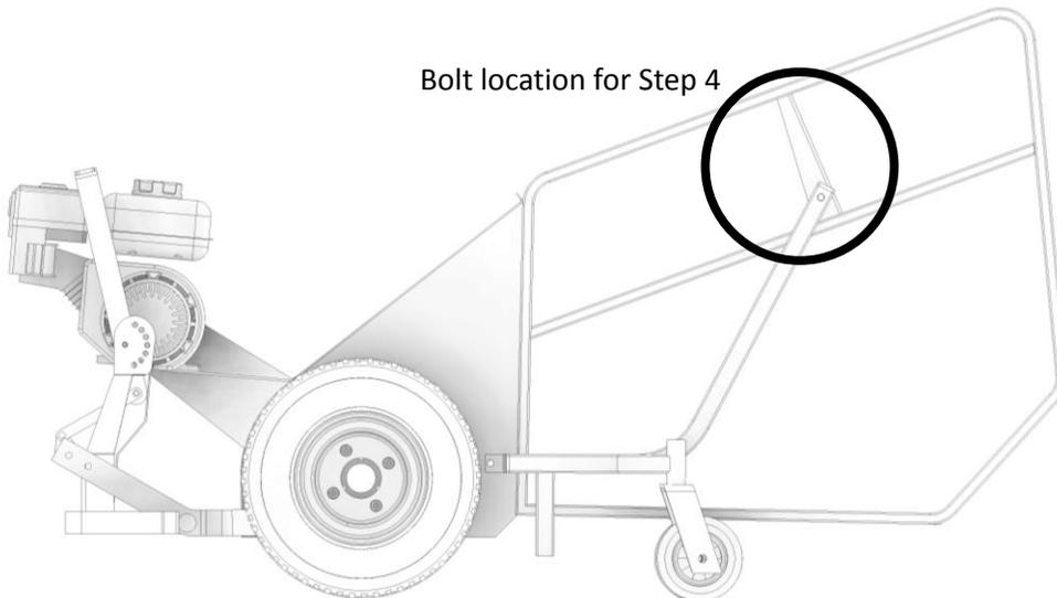
4. Fasten the hopper with the provided nuts and bolts as shown on each side.
