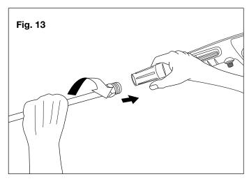
**10.** Connect the high pressure hose to the trigger gun (Fig. 14).
