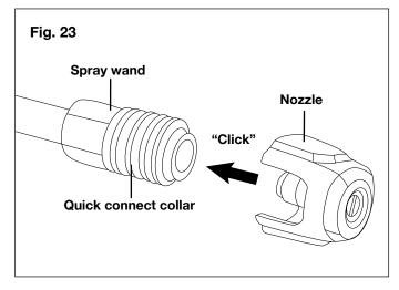
To disconnect a nozzle from the spray wand once the cleaning job is complete:
