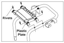
**STEP 5:** Attach the plastic plate from the top aligned to the four holes placed on top of the handle and insert the rivets through holes of plastic plate.
