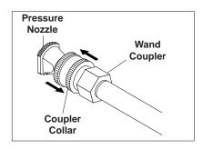
**STEP 9:** Release the coupler collar and push the nozzle until the collar clicks. Pull the nozzle to make sure it is seated properly.
