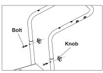
**STEP 2:** Insert the carriage bolt through the holes from the front of the unit and attach a knob from the back of the machine. Tighten Knobs with your hands.
