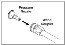
**STEP 8:** Pull spring-loaded collar of the wand coupler back to insert your choice of pressure nozzle.
