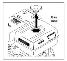
**STEP 3:** Fill gas tank with unleaded gasoline. Do not use leaded gasoline.
