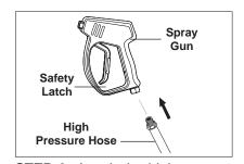
**STEP 6:** Attach the high pressure hose to the spray gun using teflon tape on hose threads.
