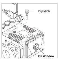
STEP 2: Remove shipping cap and install oil dipstick. Check pump oil level by using dipstick or observe oil level in oil window (if equipped). Use 40 wt. non detergent oil. The Legacy Axial Pump does not require maintenance. Attemping to check oil on this pump may damage it and will void your pump warranty.
