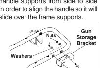
**STEP 4:** Attach the gun storage bracket and insert bolts from the outside, place washers through bolts from inside and insert nuts from inside as well. Tighten nuts.
