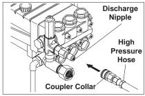
**STEP 10:** Connect the high pressure hose to the discharge nipple. Push coupler collar forward until secure.
