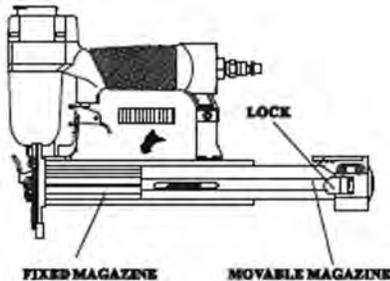
2) Place a full clip of the specified type and size fasteners on the fixed magazine, up to 100 fasteners may be loaded in the magazine.
