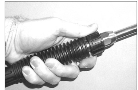
Figure 6 - Attach lance to gun
