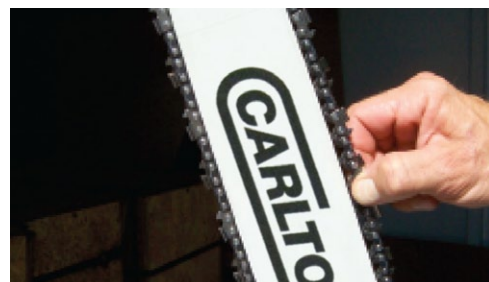
Correct chain tension.
