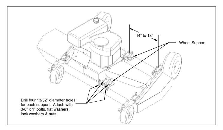
Figure 1: Installation of wheel supports
