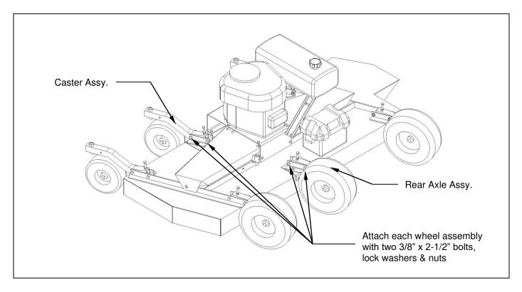
Figure 2: Installation of caster assemblies and rear axle assemblies
