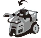
Orientate the handle assembly as shown.
