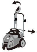
• Close for storage: Pull out on the locking pin at base of handle. Fold handle bar forward to front of unit.
