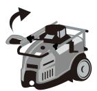
• Open for use: Lift up on the handle bar pivoting it towards the back into an upright position until it clicks and locks into place.
