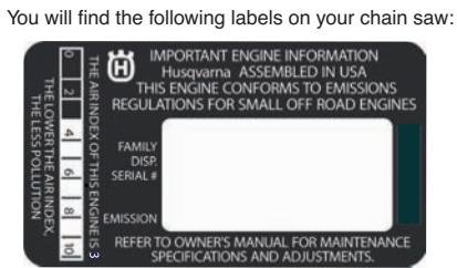
The Emissions Compliance Period referred to on the Emission Compliance label indicates the number of operating hours for which the engine has been shown to meet Federal emissions requirements. Category C = 50 hours, B = 125 hours, and A = 300 hours.
