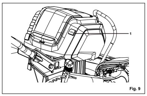
Press this button, the indicating light will be on and the mower will be in the high-speed. You can mow more efficiently when the grass is very thick.
