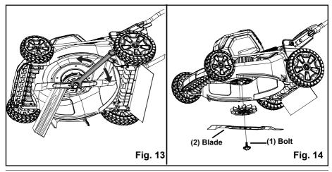
NOTE: Be sure to replace the parts in the exact order in which they were removed. When installing the cutting blade, verify that it is installed with the curved ends pointing toward the mower deck, and not toward the ground. Refer to the schematic drawing on page 34 of this manual.
