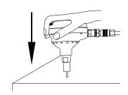
Continue to apply pressure until fastener is driven completely or until reaching desired penetration.
