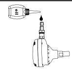
3. After adding oil, run too briefly. Wipe off any excess oil from the cap exhaust.
