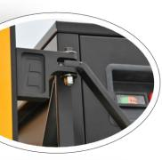
Patented swing arm mount for quick and easy maintenance, simply take out the pin and swing the dryer to the side accessing the door panel.
