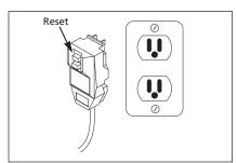
Figure 4 - Grounded plug/reset button
