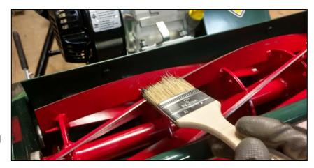
➤ Continue rotating the blade for 3-5 minutes or until the compound texture become smooth and lighter in appearance. Also note that the sound of the reel rotating against the bed knife will change as the compound texture changes.
