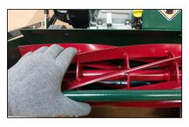
➤ Once the chain is off, you can rotate the reel blade by hand to see, hear and feel it's contact with the bed knife. It should move freely with light or no contact with the bed knife.
