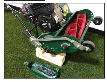
The best option is to place the entire unit on a sturdy work bench with a large surface area. If that's not possible, it's recommended that it be elevated as much as possible off the ground to provide a better view of the reel blade / bed knife point of contact and perform adjustment or back-lapping. A sturdy base (4-5" wide and in height) that the rear wheels can be placed on, will make it easier to see the blade / bed knife contact point when the unit it tipped backwards.
