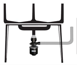
For installation on a twin laundry tub, the pump has to be centered as per this diagram.
