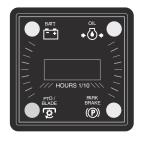
most digit). The monitor also has four indicator lights that show the status of various functions of the tractor.
