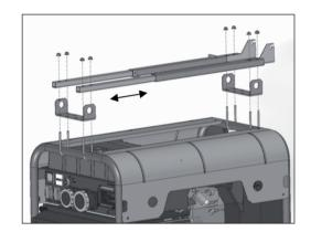
Assembly the bearing collar on the mast body. The fixing position may vary and depends on the generating set in your hands, in order to grant a safe grip of the support feet to the ground.
