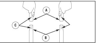
**NOTE:** It may be necessary to move the handle supports from side to side in order to align the handle so it will slide over the handle supports.
