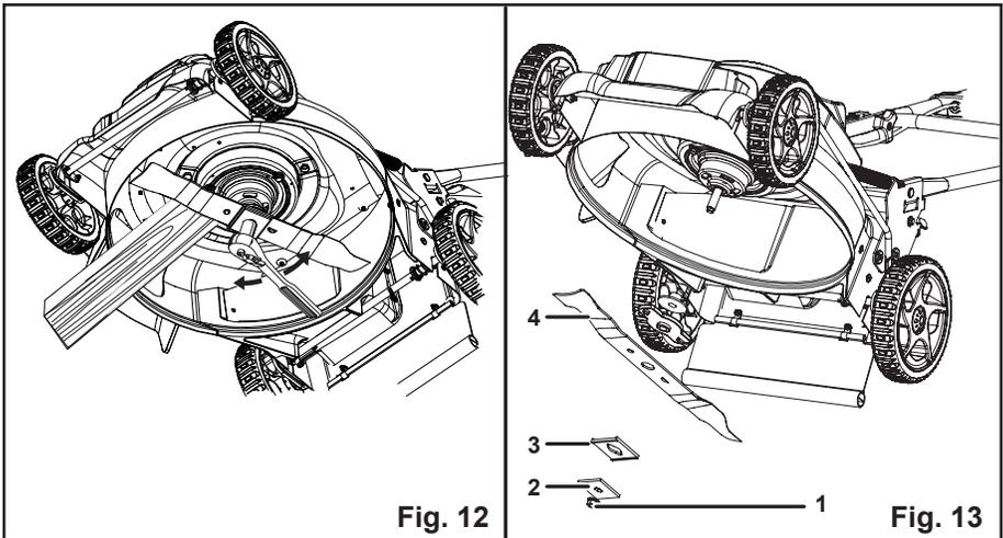
**NOTE:** Be sure to replace the parts in the exact order in which they were removed. When installing the cutting blade, verify that it is installed with the curved ends pointing toward the mower deck, and not toward the ground. Refer to the schematic drawing on page 32 of this manual.
