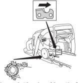
Make sure that the edges of the cutting links are facing forward on the top edge of the bar.
