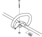
• Slide the spacer into the slot in the loop handle. Fit the nut and screw. Tighten.
