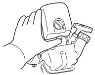
Choke: Set the choke control in the choke position.
