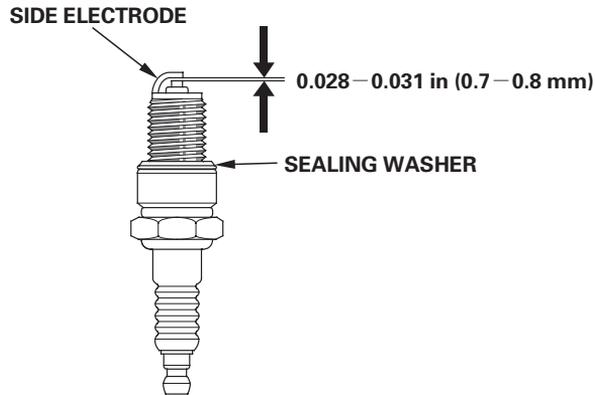
5. Check that the spark plug sealing washer is in good condition, and thread the spark plug in by hand to prevent cross-threading.
