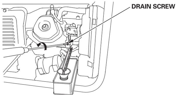
4. After all the gasoline has drained into the container, tighten the drain screw securely.
