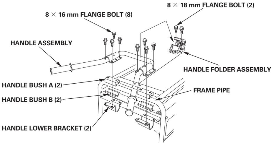
Operation must be checked after attaching the handle.
