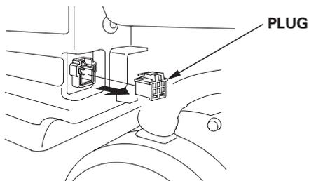
2. Connect the remote control cable to the back of the control panel and remote control box.
