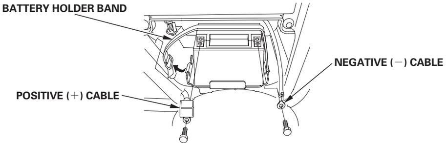
4. Remove the battery from the battery tray.
