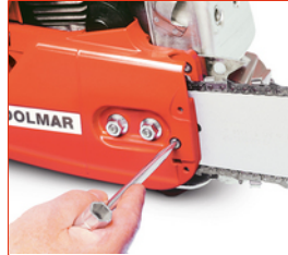
Lateral chain tensioning
