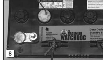
8. Rinse and dry the YELLOW cap from the old battery to remove any residue. Replace the BLACK battery cap in the cell that is 2nd from the POSITIVE post with the YELLOW cap from the old battery. Insert the fluid sensor in the cap. Put the BLACK battery cap on the old battery.
