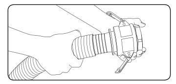
4. Fasten the quick coupler to the suction hose with the hose clamp.
