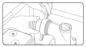
2. Slide the flexible, outlet hose over connector and secure with the hose clamp.
