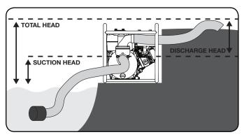
Pump output will be affected by the type, length, and size of the suction and discharge hoses. The pumping height, also known as the total head, is the distance from the water level to the point of discharge. As this distance increases, pump output decreases. The discharge capacity is greater than the suction capacity. Therefore, it is important that the suction head is less than the discharge head.
