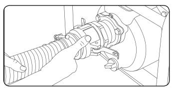
7. Attach the strainer to the intake hose and secure with the hose clamp.
