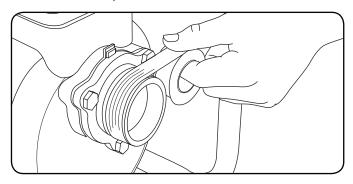
6. Attach the quick coupler to the male coupler and lock in place with the cam lock.
