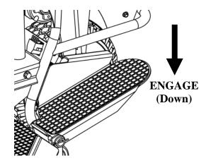
Before driving, check the direction of the drive wheel is in the direction that will drive the machine FORWARD (see Owners Manual for reference). To begin driving, depress the drive pedal all the way down until the machine begins moving forward.
