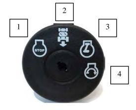
To start the machine set the throttle to fast and engage the choke. Turn the Ignition Key to position four until the engine fires. Disengage the choke after engine is running. NOTE: To mow in a generally rearward direction, turn the key to position two. To turn off the engine return the key to position one. 5
