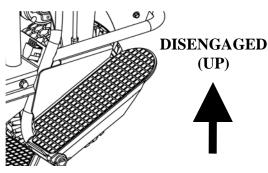
Before attempting to operate or work on the machine, be sure that the drive pedal located at the lower right side of the machine is fully disengaged in the UP position.
