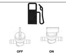
Add gas to fuel tank. Turn fuel valve to the ON position.
