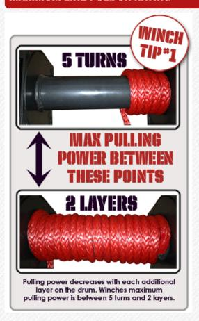
This is the maximum effort that the winch can exert on a single line on the first layer of the winch drum.
