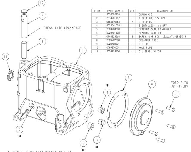
★ INSTALL WITH PIPE THREAD SEALANT
